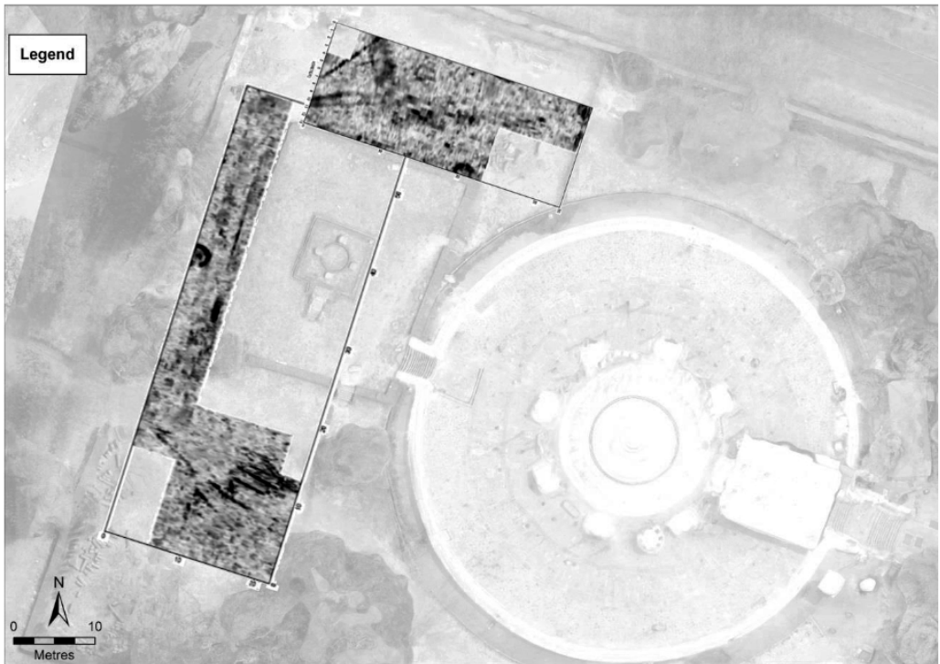
Figure 3. Results of GPR survey in Area 2 (at 3ns) and Area 3 (at 1ns).
