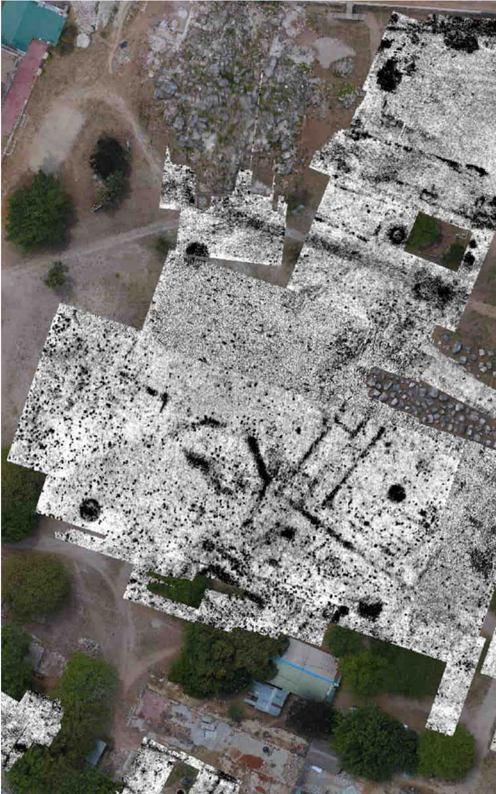
Figure 3: Detail of GPR survey results within Jaffna Fort
