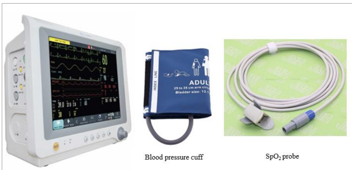
Figure 1 Lutech Datalys 760 Multipara Patient Monitor along with its components: the blood pressure cuff and the SpO 2 probe used for collecting PPG signals, oxygen saturation, pulse rate, and blood pressure for the study.
