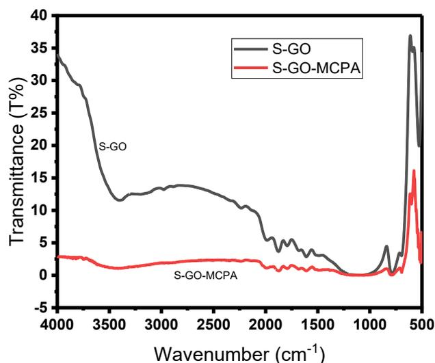
**Figure 5.** Overlapped FT-IR spectrum of M-GO/S before (S-GO) and after MCPA adsorption (S-GO-MCPA) under the optimum conditions.
