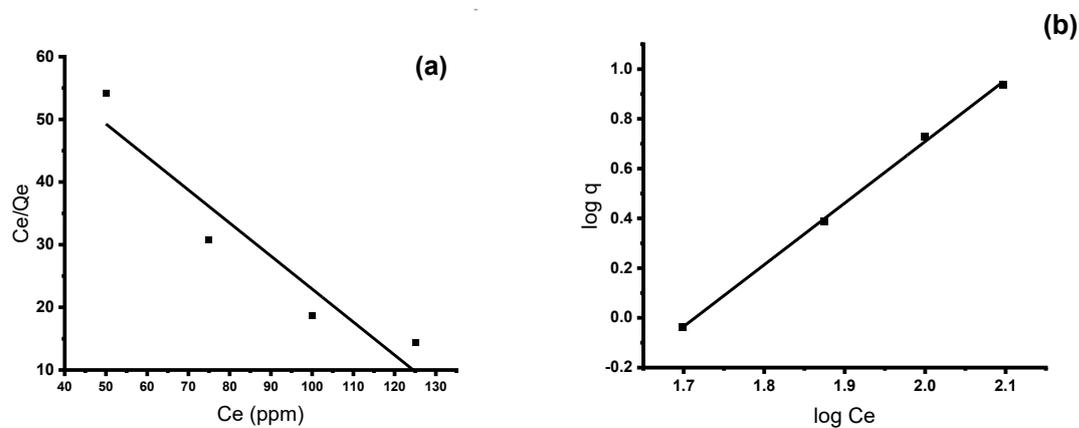
**Figure 3.** (a). Langmuir adsorption isotherm of MCPA sorption (adsorbent dose = 0.05g, contact time = 105 Minutes, initial concentration = 50 –150 mg L<sup>-1</sup>, agitation speed = 120 rpm, T = 25±2 °C) ( $R^2 = 0.995$ ), (b). Freundlich adsorption isotherm of MCPA sorption (adsorbent dose = 0.05g, contact time = 105 Minutes, initial concentration = 50 –125 mg L<sup>-1</sup>, agitation speed = 120 rpm, T = 25±2 °C) ( $R^2 = 0.9987$ )
