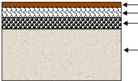
A – Neem, B – Limestone, C – Charcoal, D – Sand
