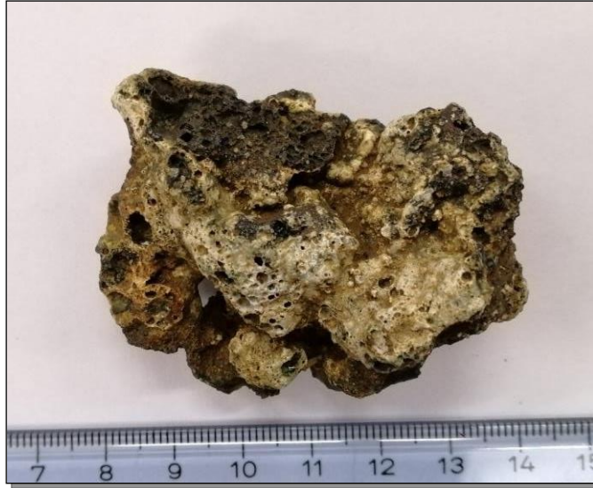
Fig.04 Slag including \text{CaCO}_3 . Scale in cm, Images and data Copyrights: WMTB Wijepala
