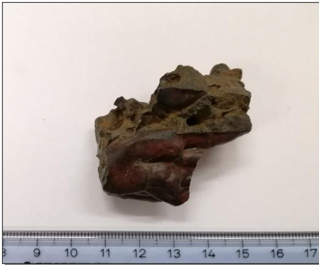
Fig.03.Red Smooth flaw-type wavy slag. Scale in cm, Images and data Copyrights: WMTB Wijepala
